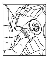
8. Put the wheel nuts back on with the rounded end of the nuts toward the wheel. Tighten each wheel nut by hand until the wheel is held against the hub.
